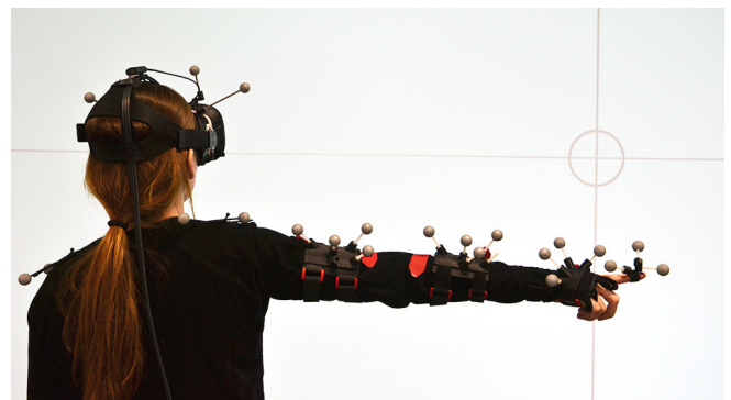
Figure 2. The seven rigid body markers used for body tracking in our study.
