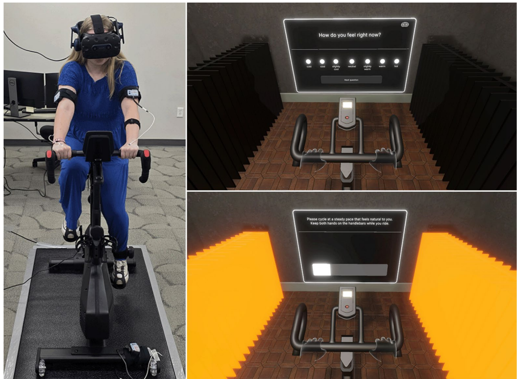
Fig. 1. Left: Participant cycling on the stationary bicycle while wearing a VR device (HTC Vive Pro 2), skin temperature sensors attached to the back of both hands (BIOPAC skin temperature thermistors) connected with transmitters (BioNomadix SKT Transmitter) wrapped around the left and right upper arm. In addition, participants were wearing a heart rate sensor (Polar OH1) on the left forearm and an optical tracker (HTC Vive Ultimate Tracker) that was attached to their left foot to register and transfer the pedal motion onto the virtual replica of the ergometer in VR. Right: Deactivated (top) and activated (bottom) heater conditions during cycling in VR. Questionnaires were presented directly in front of participants (top) and could be completed using head movements. The screen on the virtual wall displayed the experimental progress using a slider that advanced continuously at a rate of one increment per second (bottom).
