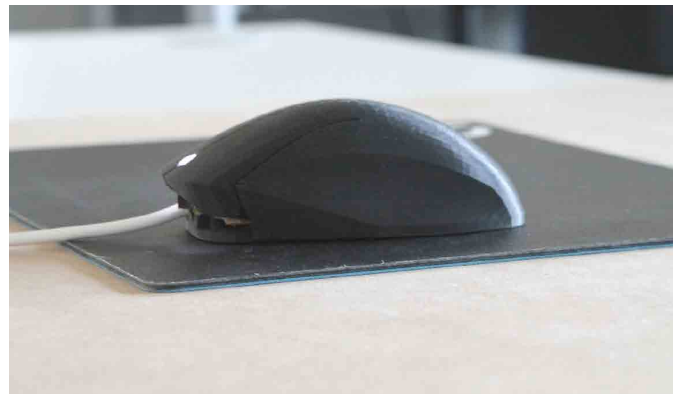
Figure 2. Rendered cross section (l.) and photo (r.) of the the 3D printed mouse. The mouse includes an optical mouse sensor, a motor for button actuation, two neodymium magnets at the front and two at the back. A LED is placed between both mouse buttons for external tracking. The robot head holds three magnets at the front, and three at the back.
